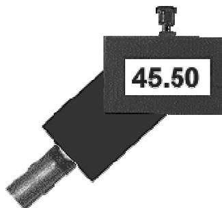
The angle of your cut is set on a protractor, or read off a digital display. How to set the angle varies slightly with the different machines. Sometimes it is a matter of loosening a setscrew, adjusting the angle, then retightening the screw. On other machines, it involves turning a handle until you reach the proper angle.
